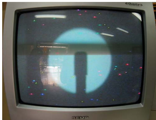
Figure 3: Radiation field and the ionization chamber images in the intensifying screen
