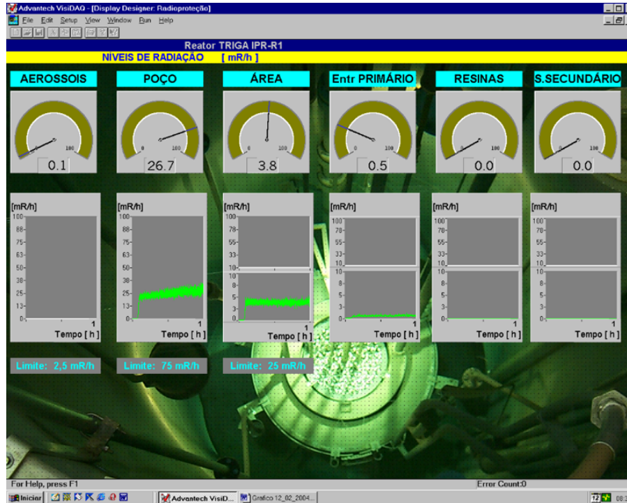
Figure 5 Radiation monitoring system
