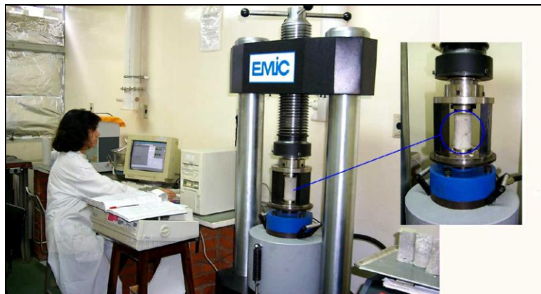
Figure 3 – Tests performed in the solidified sample of the cemented waste
