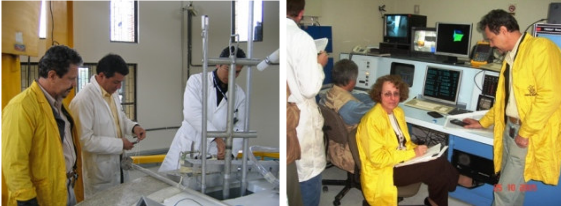
Figure 4. a) Thermal isolation of the pool before the thermal power estimation. b) The IAN TRIGA control room.
